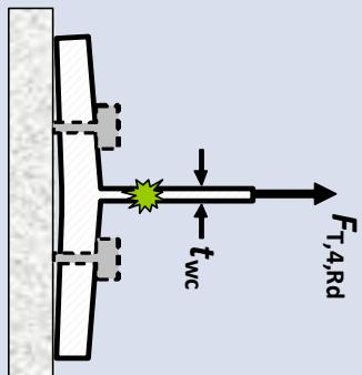
$F_{T,4,Rd} = F_{t,wc,Rd} = \frac{b_{\text{eff},t} \times t_{wc} \times f_{y,wc}}{\gamma_{M0}}$ |
